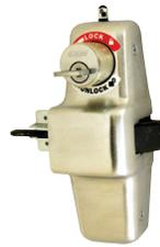
The Von Duprin Classroom Security Indicator provides an at-a-glance verification of the locked/unlocked status of the door from inside of the room. This option can be ordered as a new product or as a retrofit conversion kit to an existing 98/99 device. Indicator in Unlocked state presents a 1/2" x 1/2" metal flag (white background with black icon) at top of device head. Indicator in Locked state has no flag present.
