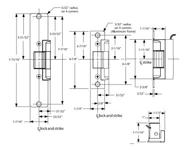
Solenoid power requirements; 12VDC, 0.38 A, 24 VDC, 0.19 A
