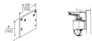
Narrow Top Rail - 88 Drop Plate: For use where a narrow top rail prevents the closer from being mounted directly to the door surface.
