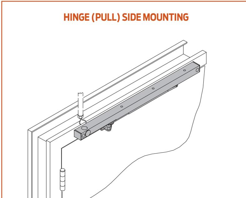
The SEH SENTRONIC® is a holder designed to provide single point hold-open for fire and smoke barrier doors that must be used with an opposite side mounted UL listed door closer. The door is held open until current interruption releases the holding mechanism and the door closes. Single lever (track) arm is specifically designed for interior doors. Choice of finishes, track functions, and installation accessories meet virtually all life safety requirements.
