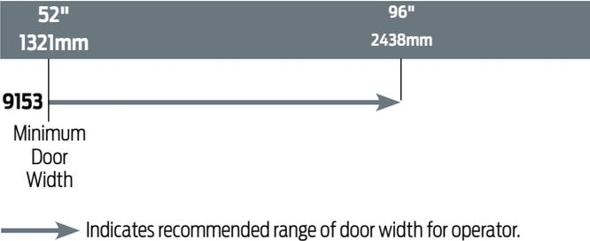
→ Indicates recommended range of door width for operator.
