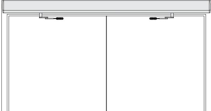
The 9150 BENCHMARK by LCN is an electrically powered low-energy operator. It provides easy access for people with disabilities, or the elderly. Designed primarily for automatic opening applications that occasionally require manual opening. The BENCHMARK is a cost-effective solution for retrofitting an activated or manual door.
