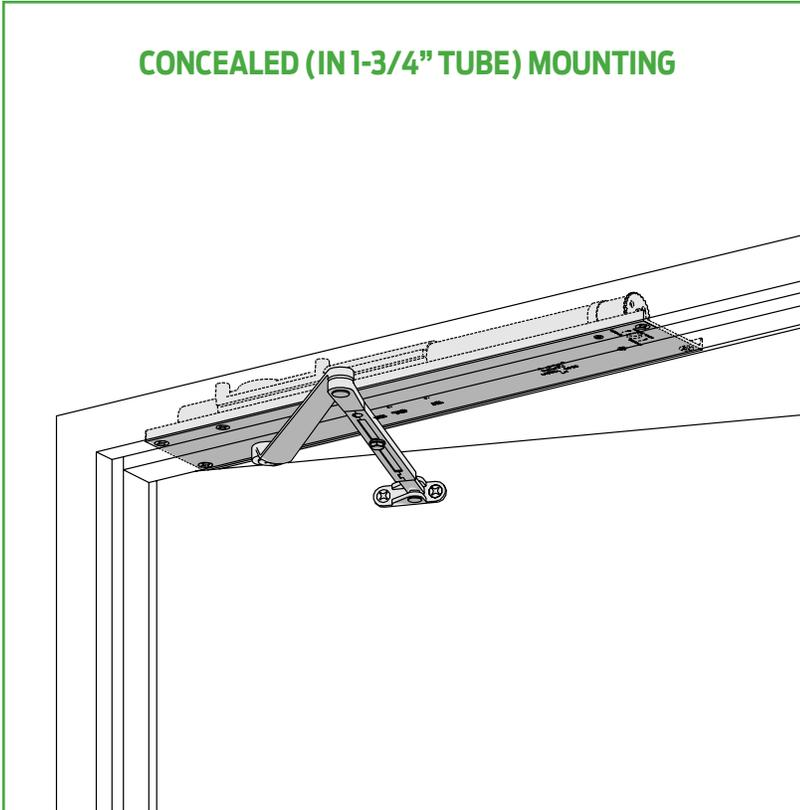
The concealed 5030 Series PACER® is a heavy duty closer designed to fit in a narrow, minimum 1-3/4" aluminum transom. The double lever arm provides superior door control and the choice of finishes and arm functions meet virtually all architectural requirements.
