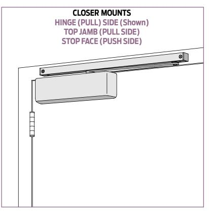
The 4040XPT is LCN's most flexible heavy duty track closer designed specifically for interior doors in institutional and other rugged high traffic applications.
