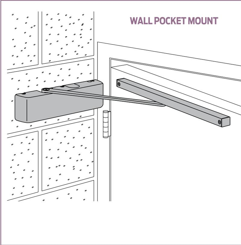
The 4000T is a heavy duty closer to reliably control fire and smoke barrier doors with maximum swing of 90°. Designed for use with an SEM 7850 wall magnet.
