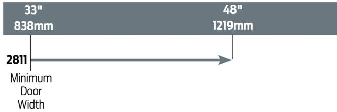
→ Indicates recommended range of door width for operator.
