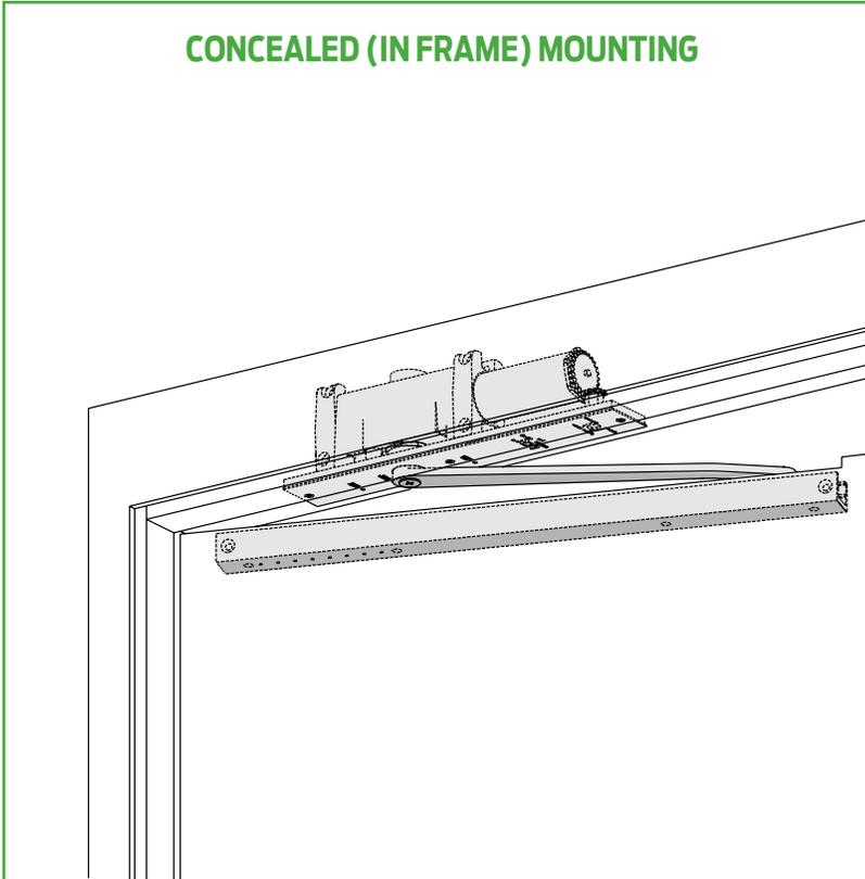
The concealed 2010 Series is a heavy duty closer designed to provide complete concealment. The single lever arm and roller assembly provide smooth, quiet door control and the choice of finishes and track functions meet virtually all architectural requirements.
