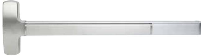
The Electric latch retraction (EL) feature provides control of latch retraction by guard or security system, allowing free entrance from outside or trim side of door. The EL system can be activated to hold the latch open momentarily or for extended periods of time, and can be interfaced with automatic doors, card readers, automatic fire alarm systems, etc.
