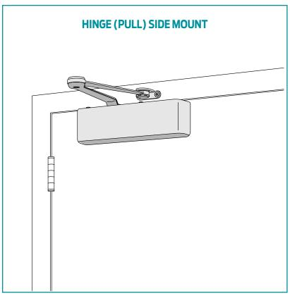
The 4510 SMOOTHEE® Series is a heavy duty, high security closer with special components to minimize tampering and vandalism. Forged steel double lever arms and heavy gauge metal security covers are designed for correctional, vandal prone, institutional and other high traffic applications. The closer has passed 10 million cycles in independent testing. A choice of finishes and cylinder functions meet correctional and vandal resistant requirements.
