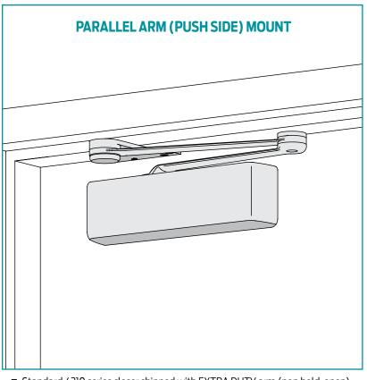
The 4210 SMOOTHEE® Series is a heavy duty, high security closer with special components to minimize tampering and vandalism. Forged steel parallel arms and heavy gauge metal security covers are designed for correctional, vandal prone, institutional and other high traffic applications. The closer has passed 10 million cycles in independent testing. A choice of finishes and cylinder functions meet correctional and vandal resistant requirements.
